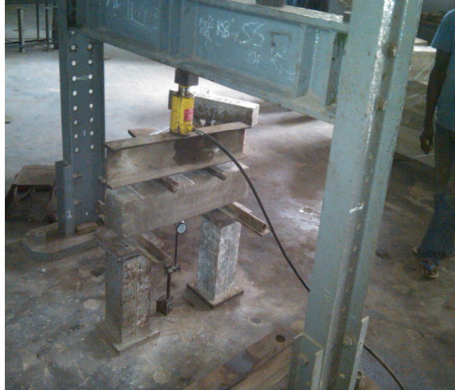
Figure 2. Testing arrangement of beam specimens
