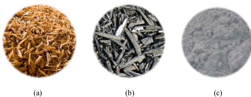
Figure 1. Rice husk (a); carbonised rice husk (b); completely incinerated rice husk (c)
