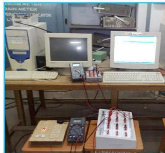
Figure 4(b). Experimental set-up for real-time implementation of adaptive controllers
