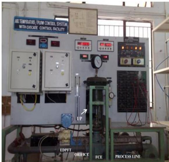
Figure 4(a). Laboratory air flow control system
