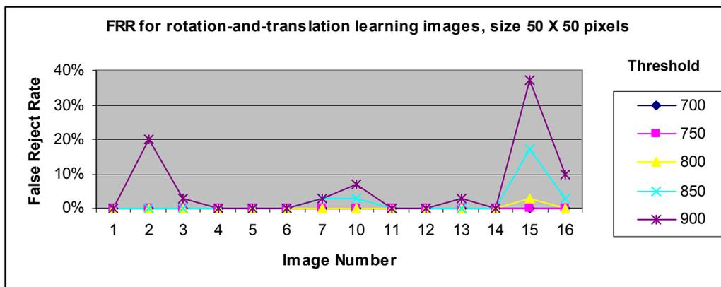
**Figure 10.** FRR for rotation-and-translation learning images, size 50×50 pixels, at various thresholds
