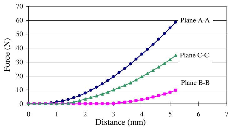
**Figure 5.** Average force-distance profiles to evaluate the critical indentation spot of fresh longan
