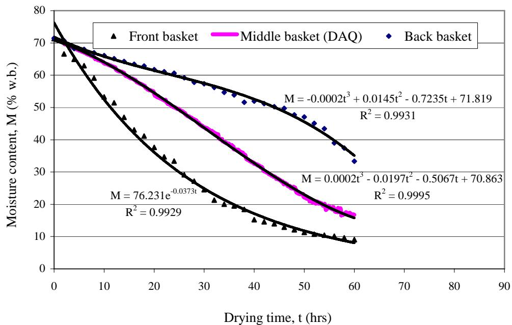
**Figure 6.** Drying curves of whole longan using hot-air (65°C) at velocity of 0.7 m/s
