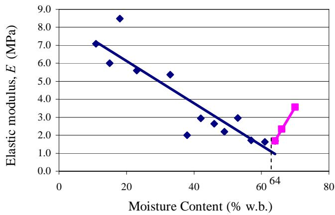
**Figure 12.** Relationship between elastic modulus ( $E$ ) and moisture content of longan
