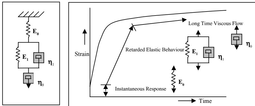
**Figure 4.** Mechanical analogy of four element Burger's model for the creep test of longan
