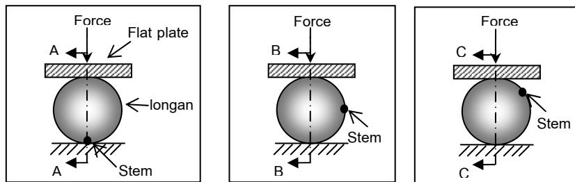
**Figure 1.** Test of critical spot of indentation on longan fruit: Plane A-A – at stem, Plane B-B – at 90° from stem, Plane C-C – at 45° from stem
