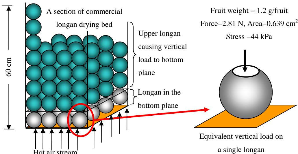
**Figure 3.** Schematic diagram of estimation of stress on longan for creep test analysis
