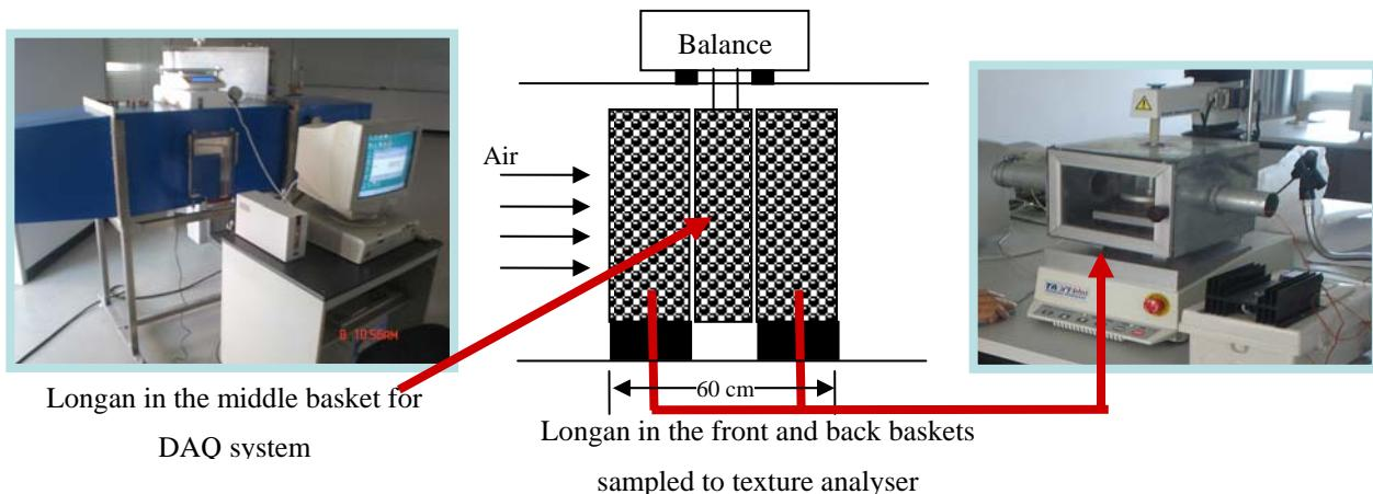
**Figure 2.** Laboratory-scaled tray dryer with DAQ system (left); Schematic diagram of longan basket setup inside drying chamber (middle); Texture analyser used for creep test (right)
