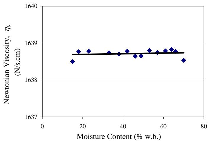
**Figure 10.** Relationship between Newtonian viscosity ( $\eta_0$ ) and moisture content of longan
