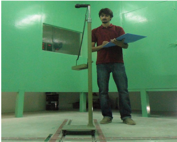
Figure 6. Stand for velocity measurement
