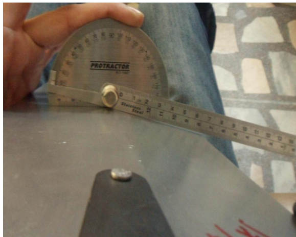
Figure 4. Bend angle measurement
