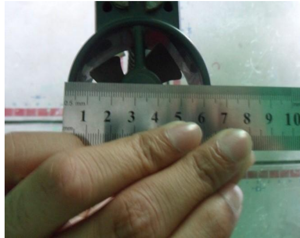
Figure 7. Diameter of anemometer sensor
