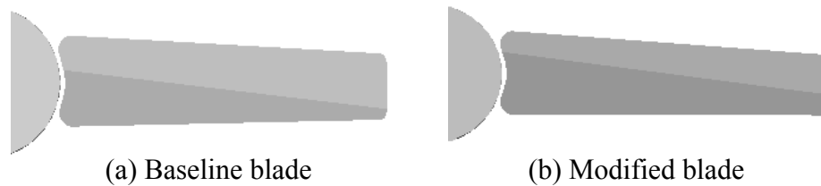
Figure 21. Comparison of baseline geometry and proposed modification of blade design
