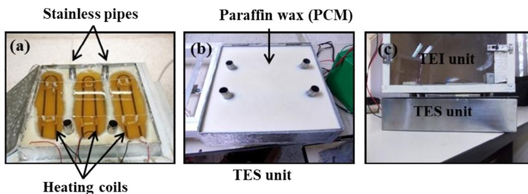
**Figure 2.** (a) 3 parallel heating elements and 2 stainless pipes inside TES unit; (b) paraffin wax contained in TES unit; (c) mounting TES unit at the bottom of TEI unit
