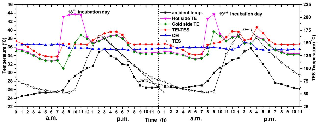
**Figure 5.** Time dependence of the temperature profiles (for TEI-TES, CEI, RT, hot and cold sides of TE module and TES) over the 18<sup>th</sup> and 19<sup>th</sup> days of incubation period
