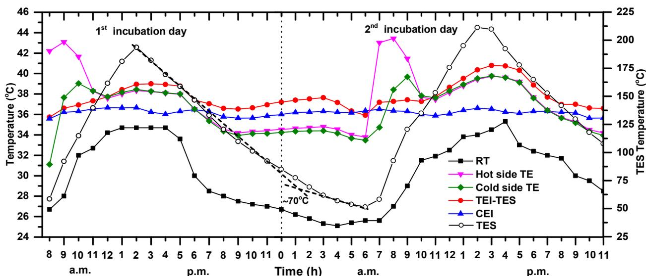
**Figure 4.** Temperature profiles over the 1<sup>st</sup> and 2<sup>nd</sup> days of incubation period of the following: TEI-TES, CEI, RT, hot and cold sides of TE module, and TES
